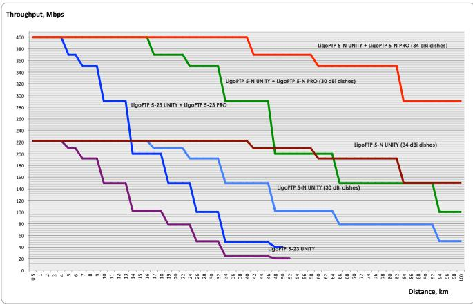
The graph above represents LigoPTP 5-23 UNITY, LigoPTP 5-N UNITY, LigoPTP 5-23 PRO and LigoPTP 5-N PRO capacity at different distances. The calculations were done with a 15 dB fade margin and no interference on
